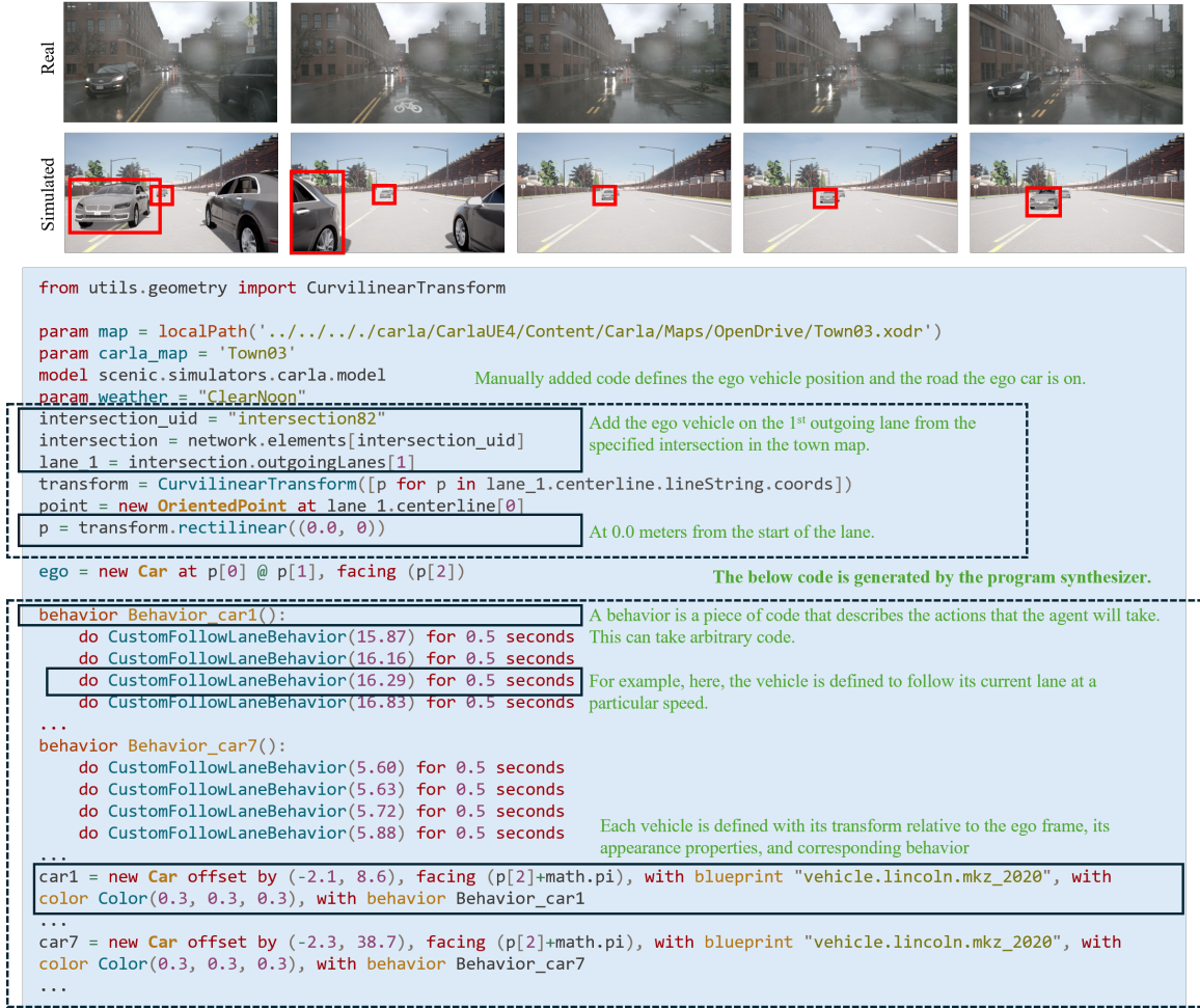
Figure 8: We present the structure of a Scenic program. A Scenic program consists of a list of specific vehicles, each with a corresponding definition. Every vehicle is paired with a behavior that describes its motion over time. The behaviors and vehicle definitions are generated by the program synthesizer.
