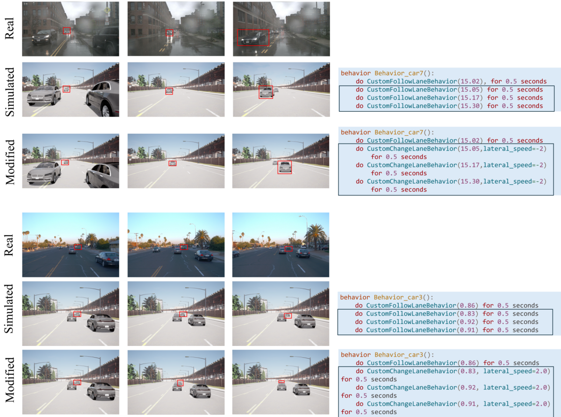
Figure 14: We show how we can manipulate the trajectory of the vehicles. We replace the instructions of a vehicle so that it performs a lane change in the simulation. The behaviors here can cause a critical situation which the autonomous vehicle must react to.
